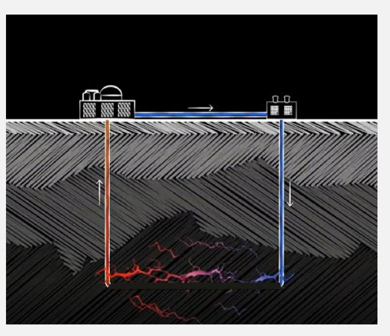
A number of production and injection wells circulate fluids through the hydrothermal or petrothermal reservoir rock formations, extracting heat for use in surface power generation facilities.
